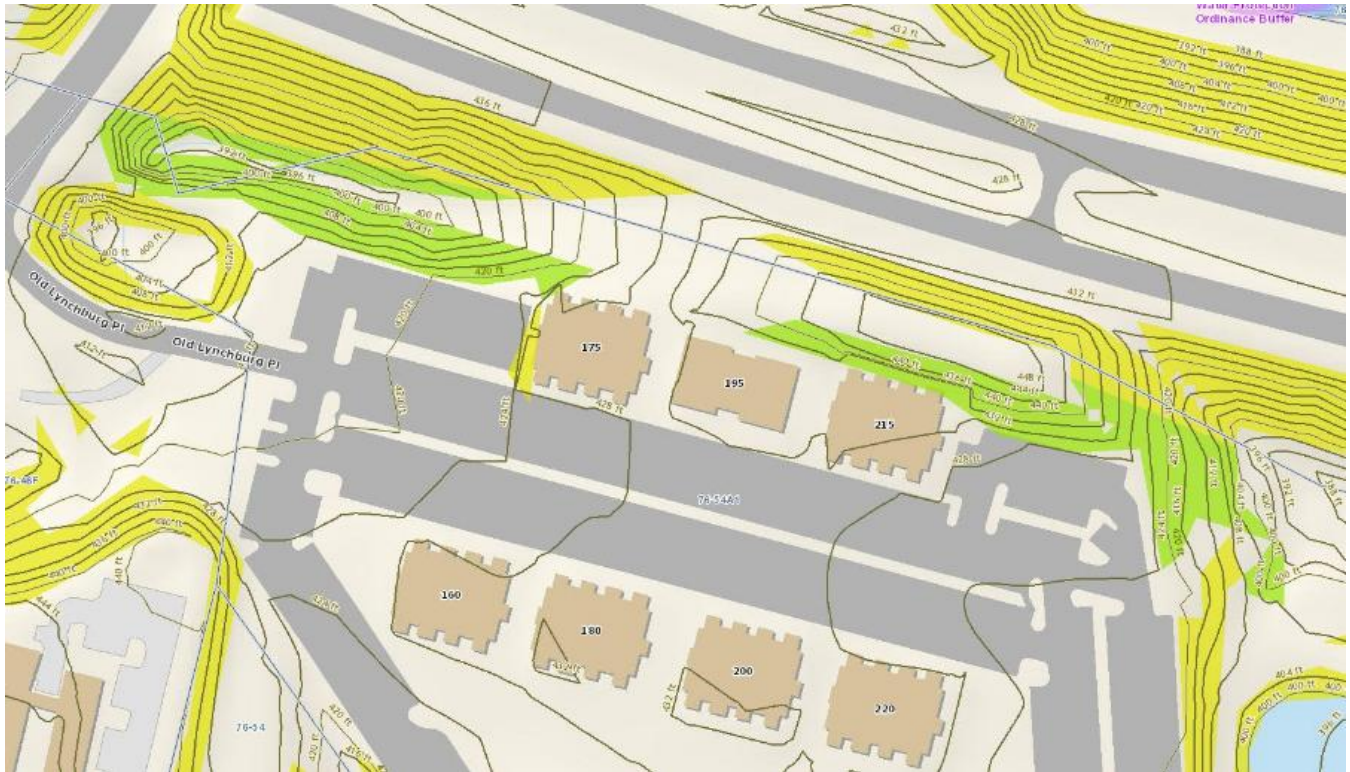
Figure 2: Steeps Slopes Overlay District on TMP 76-54A1
